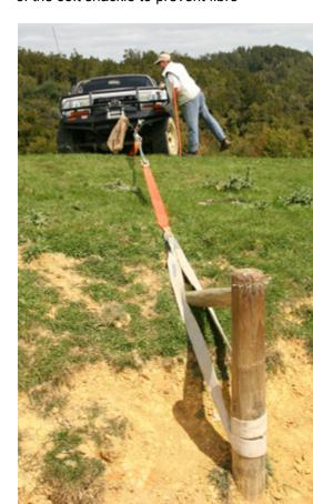
damage from overstretching the outer fibres and weakening the shackle Most of us have been in situations where we have had to double the length of a recovery strop by joining tow strops together. Again, unwanted legends have been born from the use of steel shackles to join recovery straps. There is an acceptable technique using a small length of timber between the loops of the tow straps. Get someone who is experienced to show you. It can be done relatively safely.
