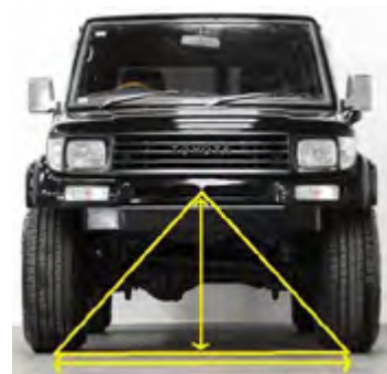
A vehicle needs a Stability Calculation when it has a body lift over 50mm; or a suspension lift over 50mm; or an increase in tyre radius over OE of more than 50mm.
